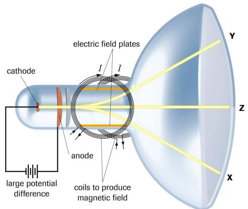
• Balancing the electric and magnetic forces allows for the straight path, Z
